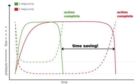
Time required to cut a typical B-pillar using a Holmatro NCT™ II cutter connected to a 2-stage or a 3-stage pump.
