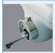
System Single-skid pick-up with spherical skid Skid radius in traversing direction 25 mm (.984"),
