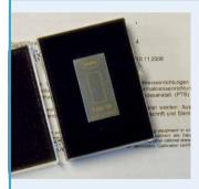
With Mahr calibration certificate. Roughness standard with turned profile, chromed. Profile depth ca. 10 µm (.394 µinch), for checking the roughness measuring station.
