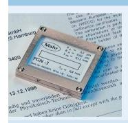
Surface standard with sinusoidal groove profile for dynamic monitoring of the roughness measuring station. Ra, Rz, Rmax. Optical flat. The following versions are available:
