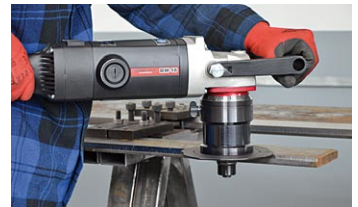
Steel plate beveling
