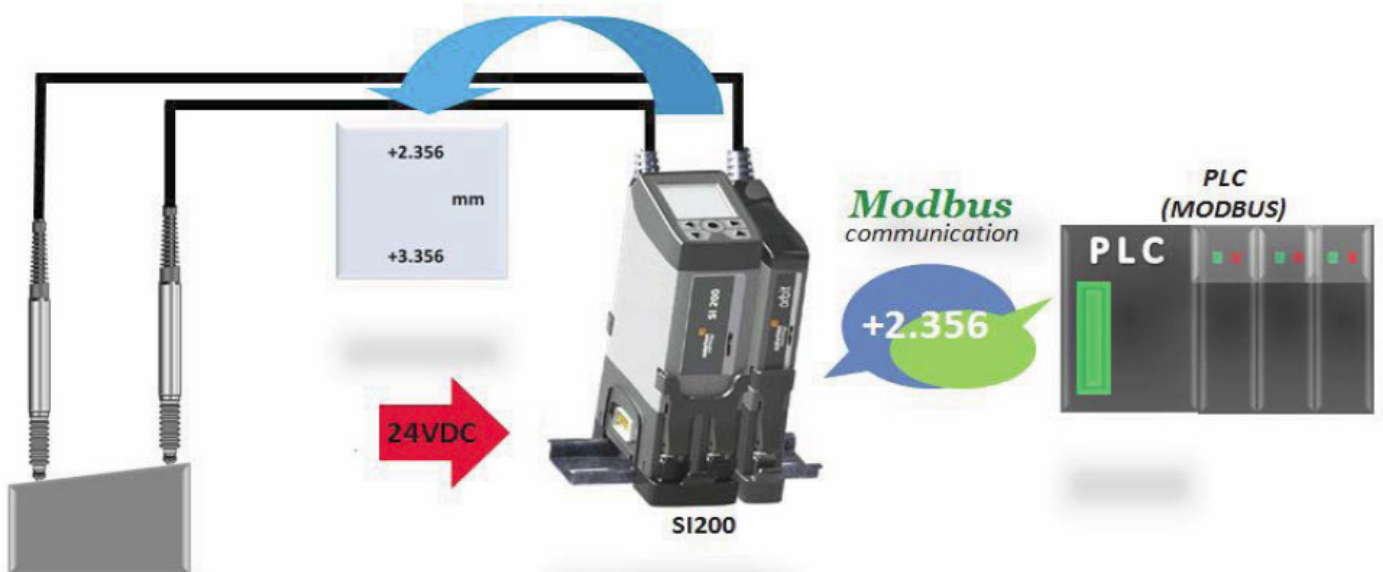
FROM MEASUREMENT SI100 to PLC via MODBUS
