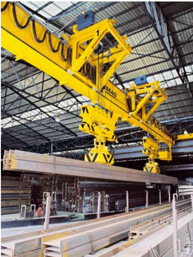
Master/slave function to synchronise motion sequences of two hoist units
